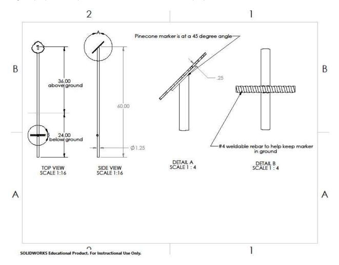
The markers currently installed on the Nature Trail were measured to be at a 40 degree angle from the ground; however, we intend to cut the pipes to be at a 45 degree angle instead (with minimal material loss). We can provide 3D-printed scaled-down models of the pinecones at various angles when our printers are available, if you would like.
