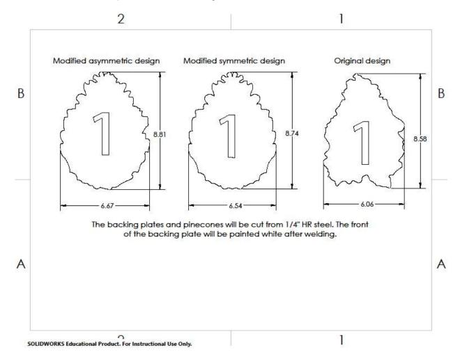
The original design was made very close to the cutouts that are currently at the Nature Trail; however, their irregular shape can make it difficult to properly cut and position both the number and the backing plate.
